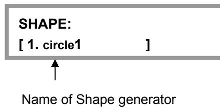
4. Press **Speed/Size** to change the Speed% and Size% value of current Shape if wanted; Indicators on.
