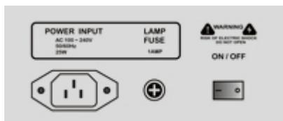
Controller adopts wide range switch power supply (AC100-240V/50-60HZ). Please confirm voltage is suitable to controller before connection. Power socket must be connected with protective groundwire to ensure safety. If to replace fuse, please disconnect power firstly and then operate to ensure safety.
