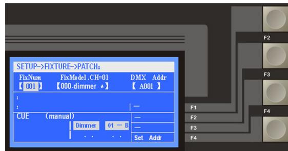
To return last layer of menu, press **BACK** key, to return Scene menu, press the current Main Menu Key once again till the flickering indicator light is off, which means returning to live show menu.
