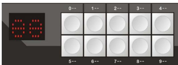
Page Turning Key locates on the right of Preset Faders. Fixture number 1~30 is in Page 0, 101~130 in Page 1, 201~230 in Page 2, 301~330 in Page 3, the rest may be deduced by analogy. Controller can also allocate the
