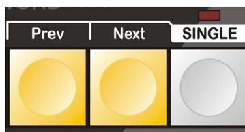
**SINGLE** —Press this key, the indicator light is on, entering the **Single-Fixture Control Mode**(control the selected fixtures one by one), press again to quit the **Single-Fixture Control Mode**.
