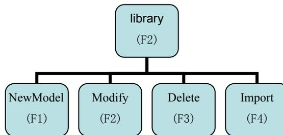
**New Model:** If fixture model needed is not in Library System, a new fixture model can be created by users. Under **Library** menu,
