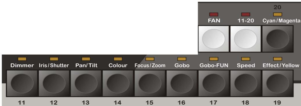
ATTRIBUTE contains 10 attribute keys, a FAN key and an “11-20” attribute switch key. Channel attribute of intelligent fixture includes Dimmer, Color and GOBO etc. Users firstly selects the attribute to be modified through attribute key and then modify the corresponding attribute through A/B wheel.
