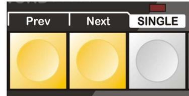
**TIPS:** Multiple fixtures can be controlled one by one after entering **SINGLE control mode**. This function is useful in programming Pan/Tilt location.
