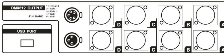
There are 4 groups (A,B,C,D) of DMX512 output sockets (shown as the above), each group contains a 3-pin XLR and a 5-pin XLR, pin one for signal ground, pin 2 for negative, and pin 3 for positive, for 5-pin XLR, pin 4 and pin 5 are blank.
